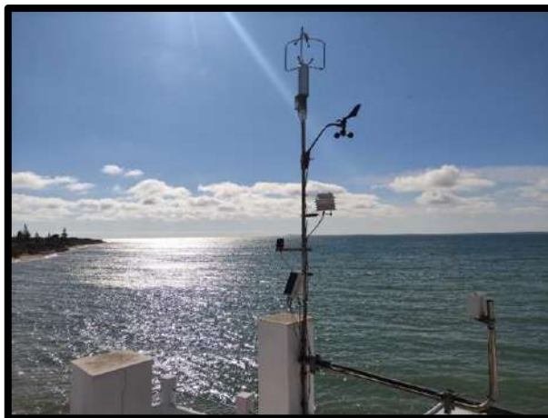
Fig. 2. Example of coastal observations that will be included in the new OceanUCA platform. In this case, the picture shows a remote automatic weather station installed in Chipiona, providing real-time data on wind speed, wind direction, temperature, humidity, pressure, and downward short-wave radiation data. Besides, this station has a 3D sonic anemometer at its top to calculate turbulence and surface heat flux data directly from high-frequency measurements (10 Hz) through the Eddy-covariance technique. These types of observations will be also included in the system.
